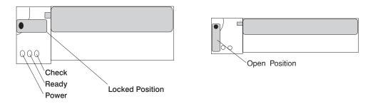
**Attention:** SSA backplanes must be fully populated. Each backplane connector must have a disk drive or a blank carrier installed at all times. If you remove a disk drive from a bay and do not replace it with another disk drive, you must install a blank carrier in that bay.
